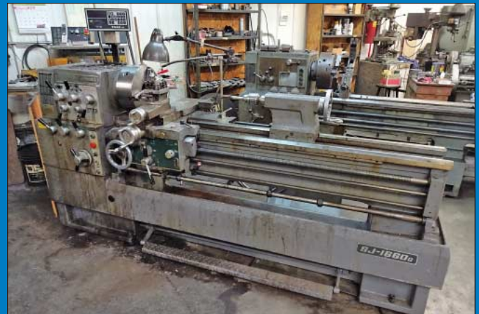
16" X 60" Millport Model SJ-1660C Geared Head Gap Bed Toolroom Engine Lathe
